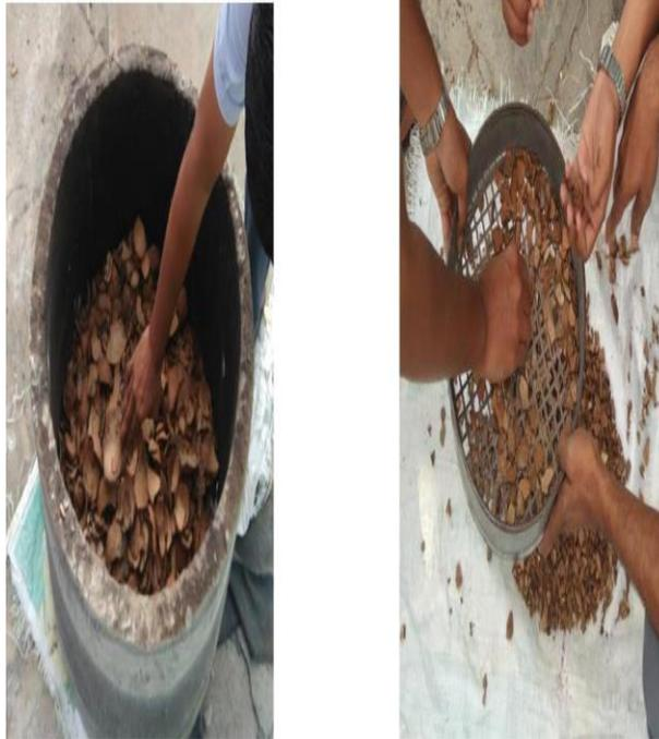
Figure 3. Breaking & sieving of coconut shells to required size.
